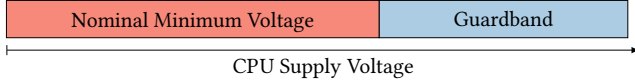
Figure 1. Typical supply voltage of a CPU. It must be higher than the nominal minimum voltage to account for all uncertainties of the CMOS circuit, aging, temperature and its surroundings.
