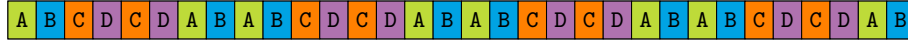
Fig. 6: The offsets within a DRAM row are parts of different memory pages A to D. Each part has the size of two cache lines, 128 bytes. This example is based on the DRAM addressing functions of a Skylake CPU [33].
